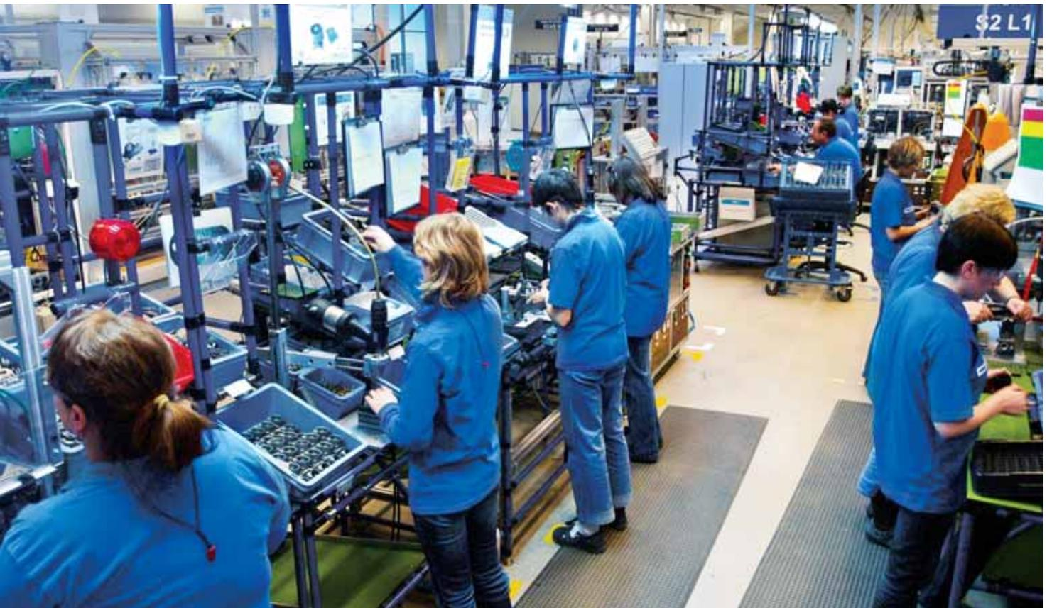
Using **LEAN MANUFACTURING METHODS** to assemble ABS modulator valves, this production line in Wrocław, Poland, combines high flexibility with the most simple and effective technical solutions. It produces for Europe and Brazil.
